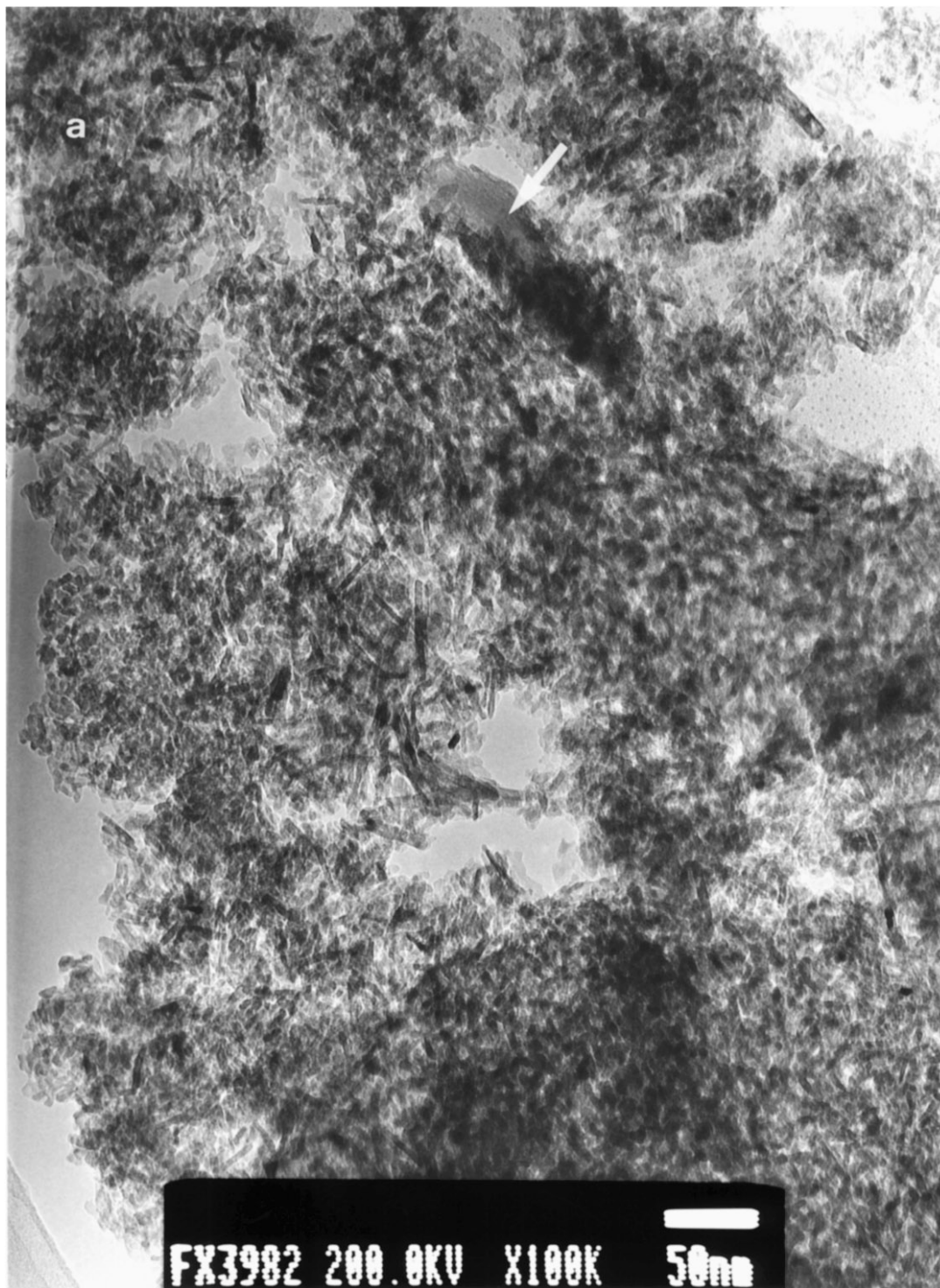
FIG. 3. TEM images for the 3% Cu/Al 2 O 3 (OH) (3a) and 5% Cu/Al 2 O 3 (H) (3b) catalysts. In 3a an arrow locates a Cu 2 O-like microcrystal (see text for details).
